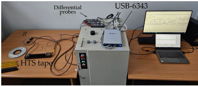
Fig. 34. Laboratory test bench for recovery time
